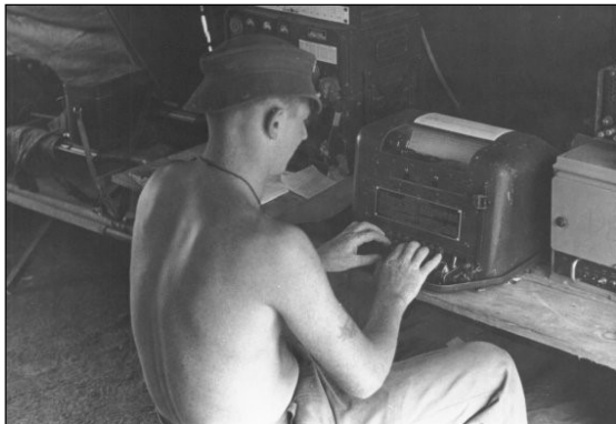
Photo 7.6 (left) - LCpl Malcolm Fergusson manning HF RTT Link - AN/GRC-106 (left), TT-4 (centre) and KW-7 (right) (1968).
