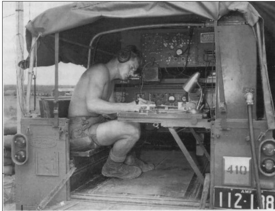
Photo 2.8 - Cpl Rex Gabel, 709 Signal Troop, transmits in morse code at Bien Hoa to HQ AAFV in Saigon. The radio set in use is the medium-power AN/TRC-75 (Sept 1965).
