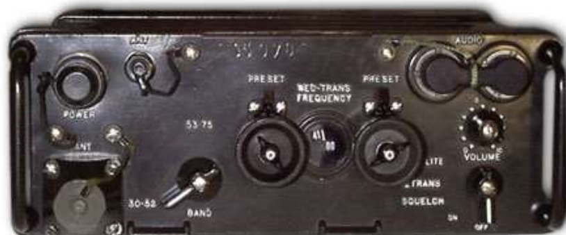
Photo 1.4 - AN/PRC-25 VHF Radio Set - Front panel layout.
