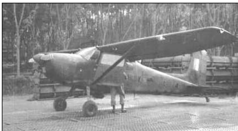
Photo 5-1.6 - Cessna 180A with ARDF equipment at Nui Dat - Note antenna pod in the up position
