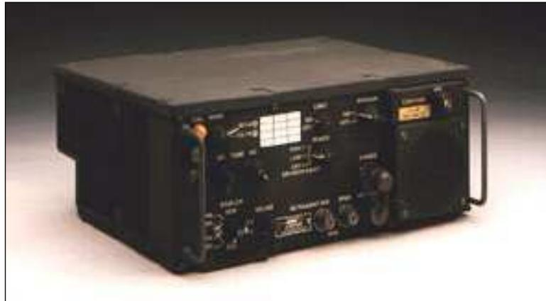
Photo 1.5 - RT-524 Transceiver (Part of AN/VRC-12 series)
