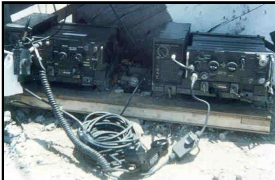
Photo 4.2 - Two AN/GRC-125 Radio Sets in retransmission configuration. Note Vehicle mounted version of the AN/PRC-25 Radio Set.
