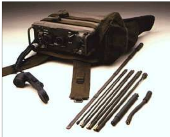
Photo 8.14 - AN/PRC-77 Radio Set with its two field Antennas.
