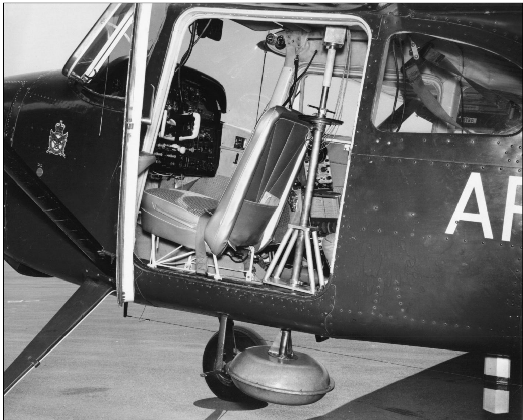
Photo 5-1.7 - Cessna 180A fitted with ARDF equipment.
