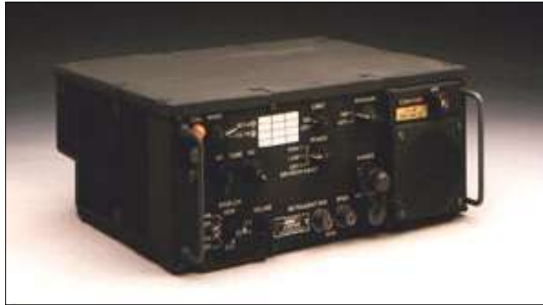
Photo 1.5 - RT-524 Transceiver (Part of AN/VRC-12 series).
