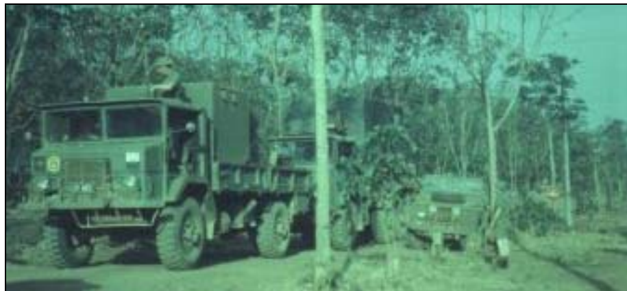
Photo 6.7 - 104 and 110 Signal Squadron vehicles at start point Nui Dat for deployment on Operation Toan Thang. Note first truck (2½ ton) AN/MTC-7 and AN/MGC-17 Shelters, second truck (5 ton) AN/MRC-69 Shelter (April 1968)
