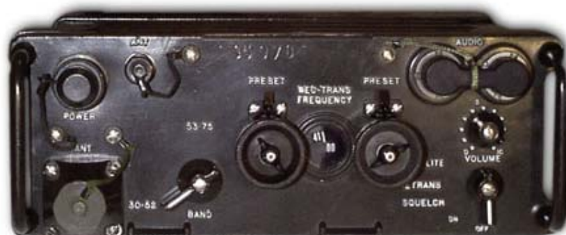
Photo 1.4 - AN/PRC-25 VHF Radio Set - Front panel layout
