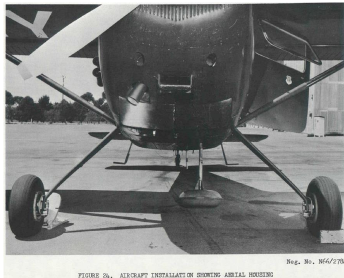
FIGURE 24. AIRCRAFT INSTALLATION SHOWING AERIAL HOUSING
