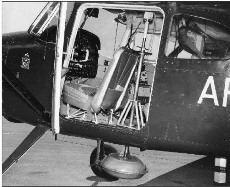
Figure 10: Prototype ARDF Equipment in Cessna 180b Aircraft
