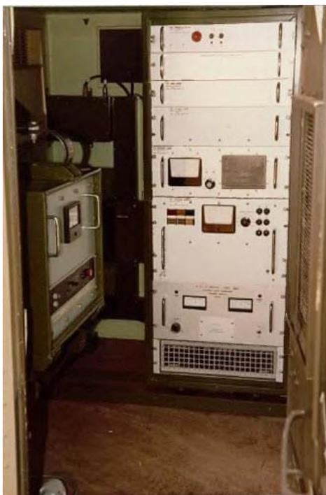
Figure 8: Ionosonde transmitter and amplifier
