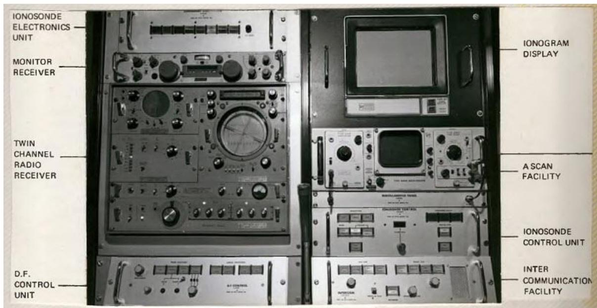
Figure 5: Part of the Operators Console
